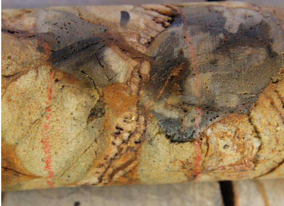
Figure 7-12 Speck of visible gold in a rusty-white quartz vein in HQ drill core (6.35 cm diameter) (NAM2017DD-004 at 78.80 m)
