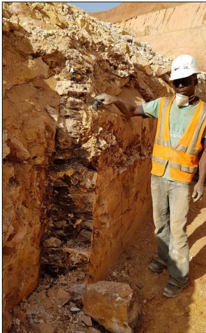
Figure 7.16 – Thick subvertical ENE-WSW en echelon quartz veins in a trench in the Central Domain. The steep dip is to the SSE.
